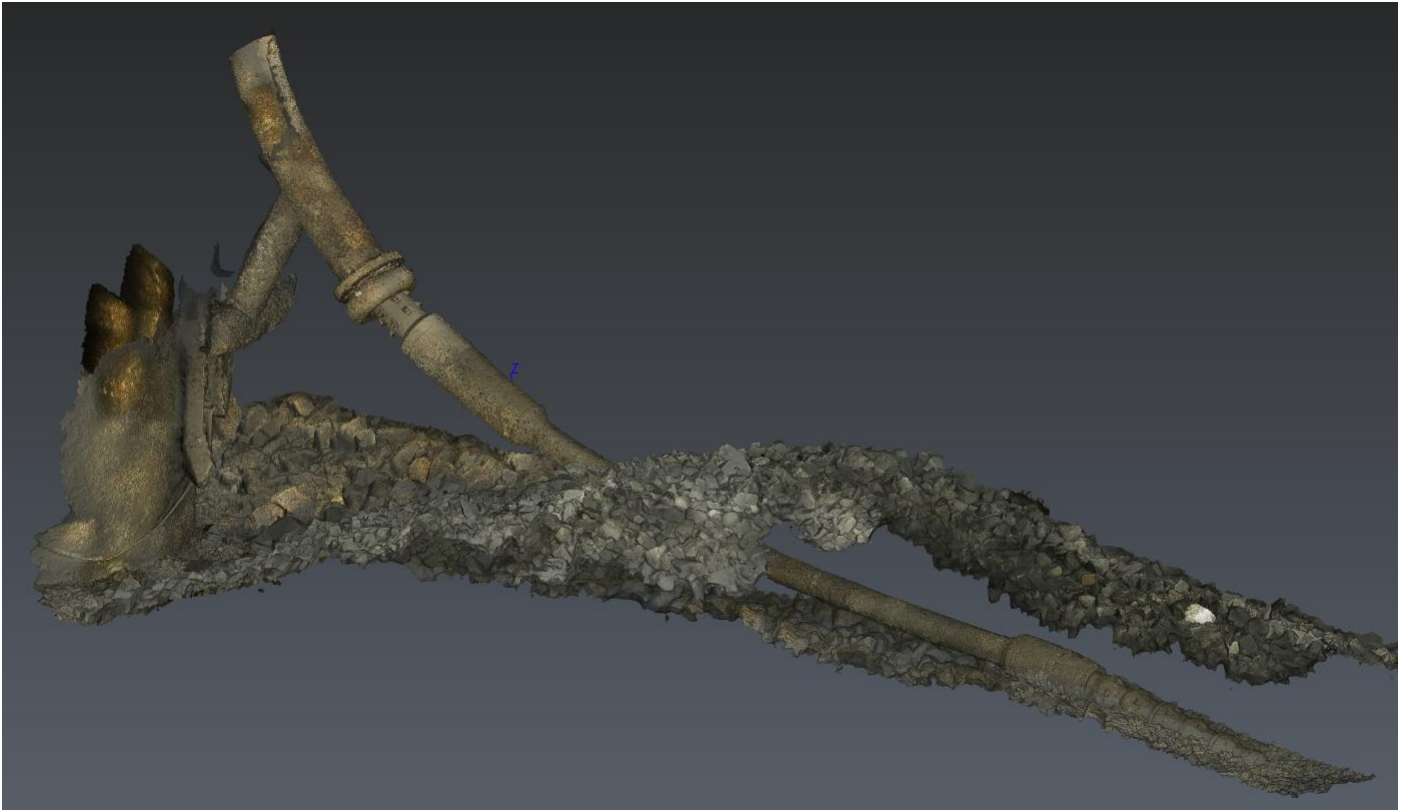
Image showing the overlay of both Mesh 3D models from phase I and phase II of the OSP East CPS cable at from touchdown to bellmouth
